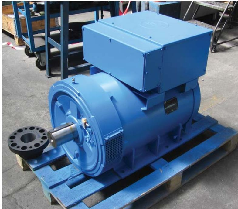
Gilbert Gilkes & Gordon Ltd (a BHA sponsoring member) supplied the 100kW 10.5" single jet Turgo turbine, fitted with a Woodward mechanical governor and flywheel. It has an Amco Marelli synchronous generator.
